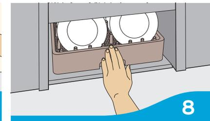
Load rack into machine and shut door. Do not remove rack until green "Cycle" light turns off.
