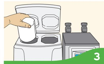
Check detergent and rinse aid. Replace if low. Make sure cover is completely shut.
