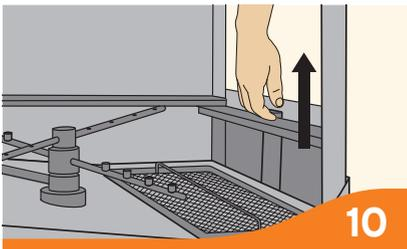
Lift drain lever and drain machine completely.
